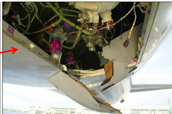
Figure No. 2: Photograph of Damage to Service Bay and Associated Structure
